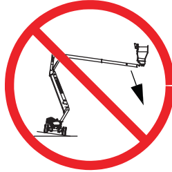
Tip Over Hazard
