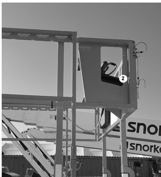
Figur 6.2 – Kontrolboksens placering, Platformposition
