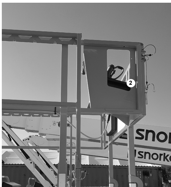
Figur 6.2 – Kontrolboksens placering, Platformposition
