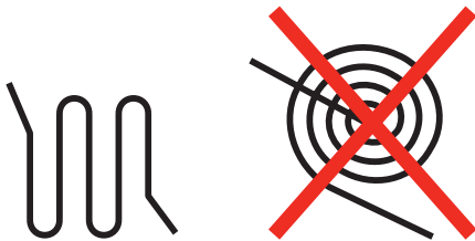
Figure 2-1 Recommended way to handle excessive cable length.
